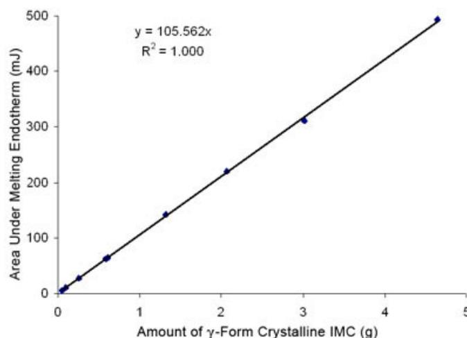
Figure 1. DSC calibration curve of  $\gamma$ -form crystalline IMC.
