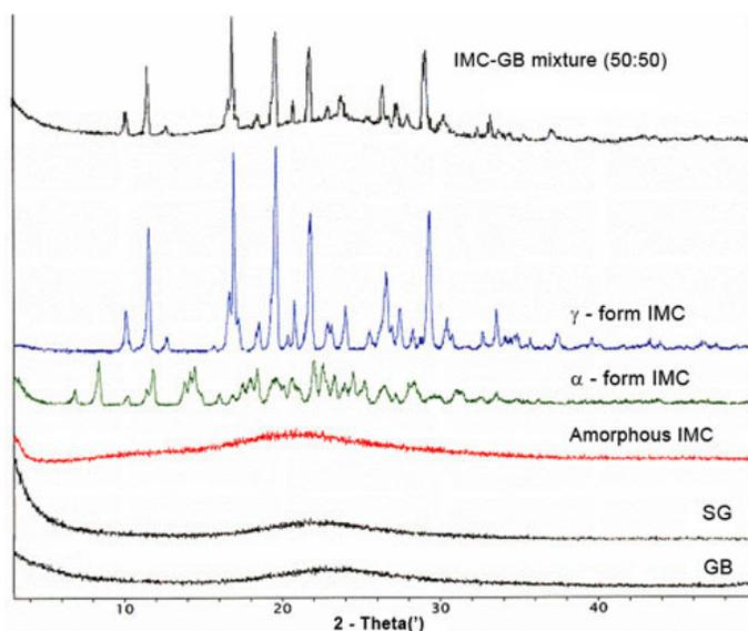
**Figure 3.** XRPD patterns of GB, SG, amorphous IMC,  $\alpha$ -form IMC,  $\gamma$ -form IMC, and IMC-GB mixture (50:50).
