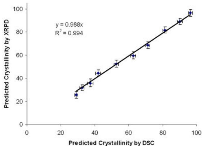
**Figure 6.** Correlation between predicted crystallinity of IMC in IMC-SG mixtures as measured by DSC and XRPD.
