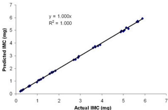
**Figure 2.** Correlation between predicted amount of crystalline IMC in IMC-GB mixtures obtained using DSC calibration curve and actual amount of IMC in IMC-GB mixtures as determined by HPLC.
