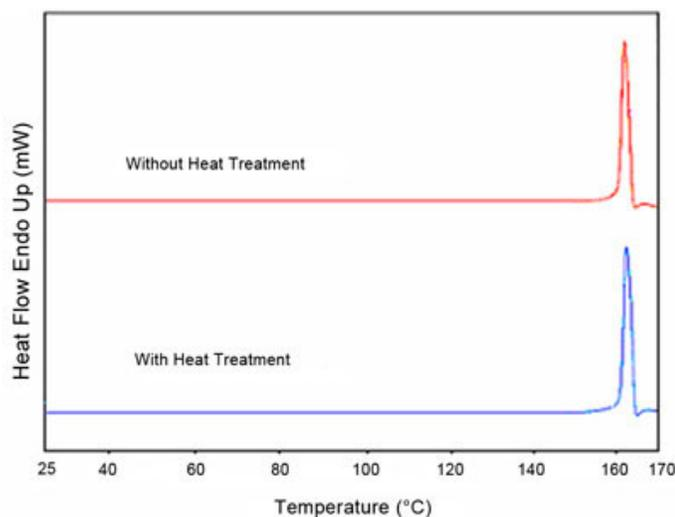
**Figure 5.** DSC profiles of IMC-SG (30:70) mixtures with and without heat treatment.
